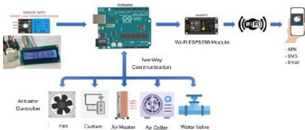
Figure 6. Equipment communication schemes and flows [18]
