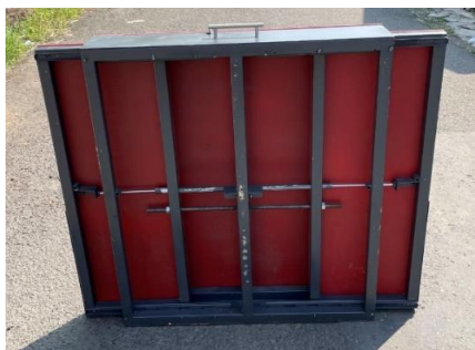
Figure 10. Flood barrier prototype
