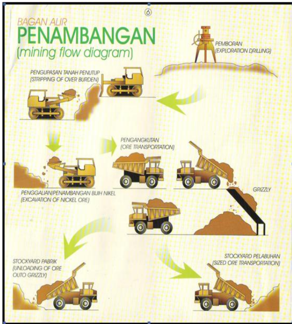
Figure 1. Scheme of nickel exploitation/mining activities. Source from a brochure PT Aneka Tambang (Persero) Tbk.
