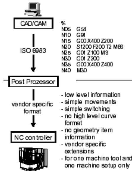
Figure 1. Current NC Programming Interface (Weck, et. al., 2001)
