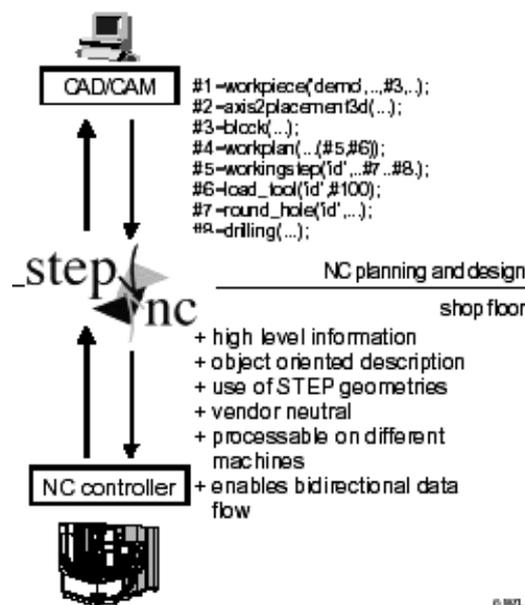
Figure 2. STEP-NC Programming Interface (Weck, et. al., 2001)
