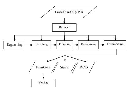
Figure 1. Production process flow of palm olein
