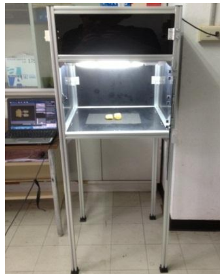
Figure 1. Image processing equipment for nugget inspection
