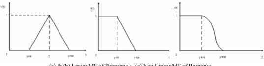
(a) & (b) Linear MF of Response ; (c) Non Linear MF of Response
