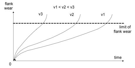
Figure 1. The Growth of Flank Wear at Some Speeds of Cutting (v<sub>i</sub>)
