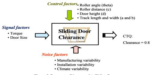
Figure 3. Parameter Diagram of A Sliding Door.
