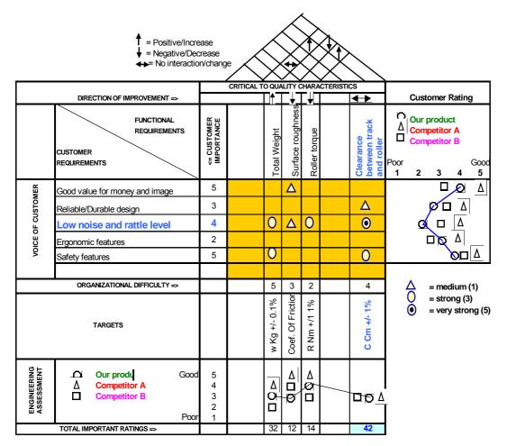
Figure 2. Quality Function Deployment of A Sliding Door.
