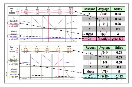
The baseline design results compared to the optimal and robust design results using Minitab Optimizer which is based on Desirability Function method are given in Figure 6.
