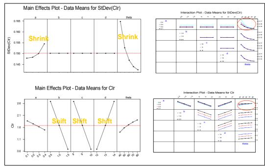
Figure 5. Main Effect and Interaction Plots of A Sliding Door DOE
