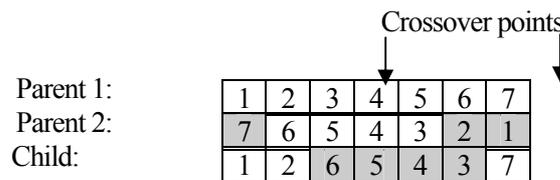
Figure 1. Two-Point Crossover combined with NEH algorithm
