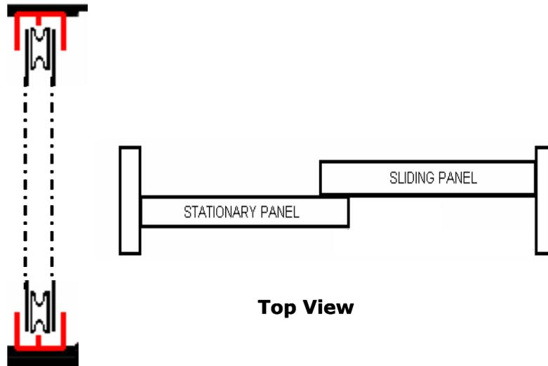
**Figure 1. Side and Top Views of A Sliding Door.**
