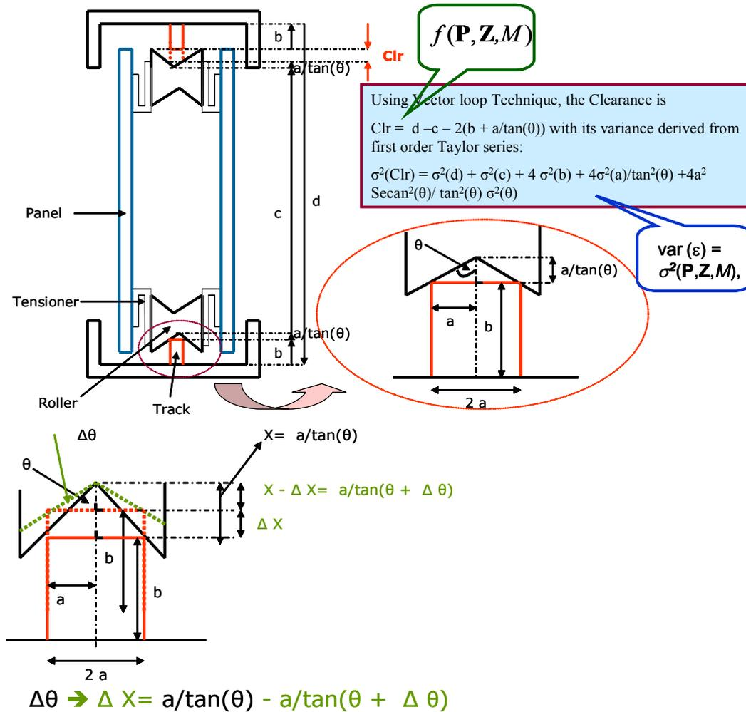
Figure 4. Transfer Function of A Sliding Door Derived From Vector Loop Technique
