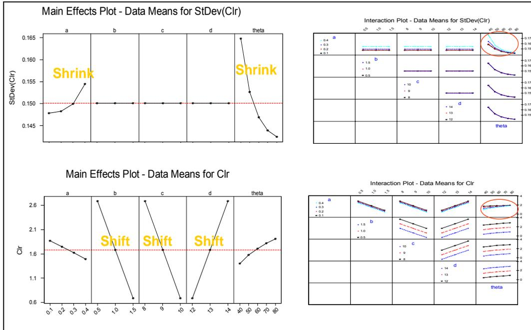
Figure 5. Main Effect and Interaction Plots of A Sliding Door DOE
