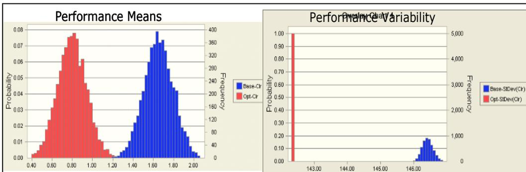
Figure 8. Monte Carlo Simulation Results of Baseline and Robust Designs of A Sliding Door.
