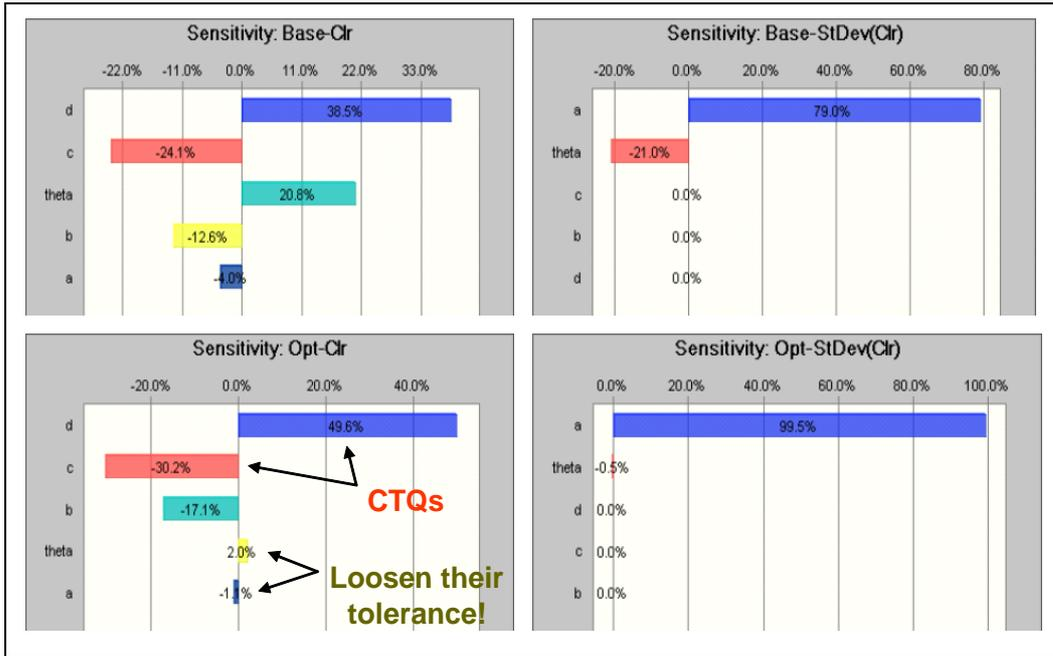
Figure 7 Local Sensitivity Analysis of Baseline and Robust Designs of A Sliding Door.
