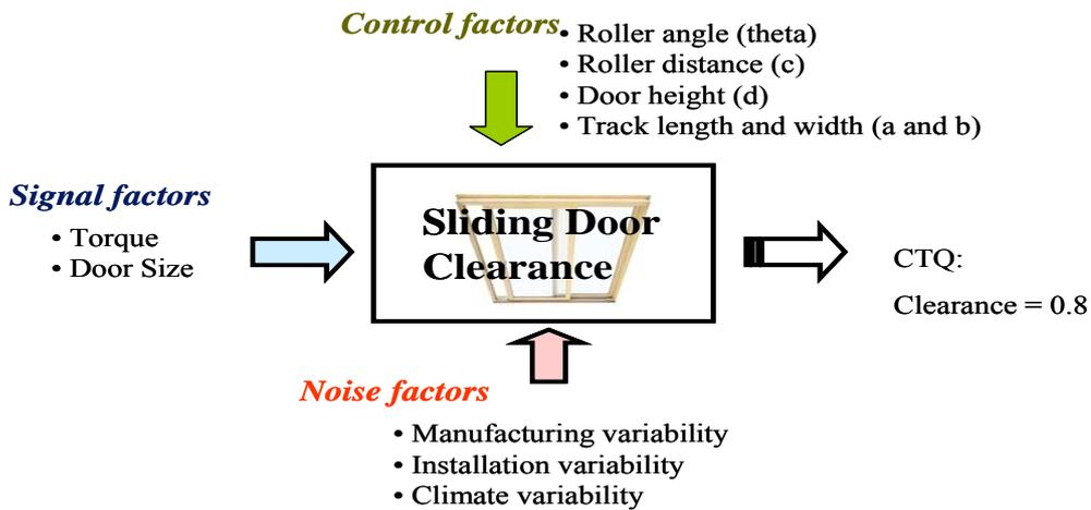
Figure 3. Parameter Diagram of A Sliding Door.
