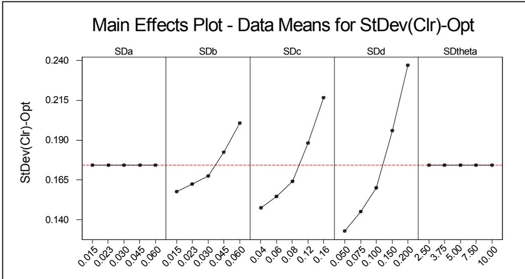
Figure 9. Main Effect Plot of Tolerance Design of A Sliding Door
