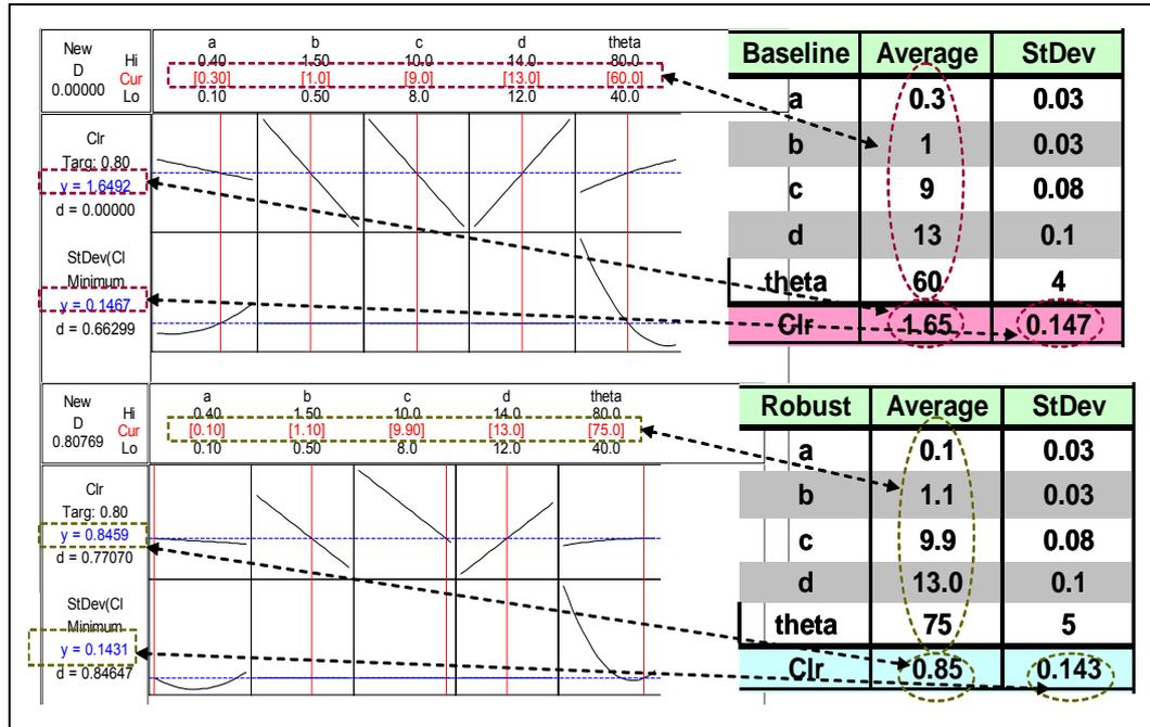
Figure 6. Baseline and Robust Results of A Sliding Door.
